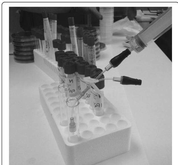
Fig. 1 Laboratory procedure for needleless connector (NC) flushing
