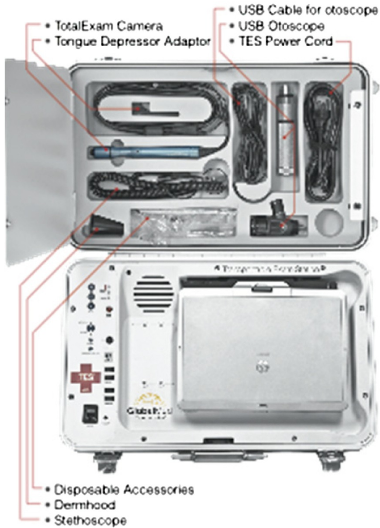
Figure 2 Miniaturized mobile telemedicine platform TES® (Transportable Examination Station; GlobalMed® Inc., Scottsdale, AZ, USA). USB, Universal Serial Bus.
