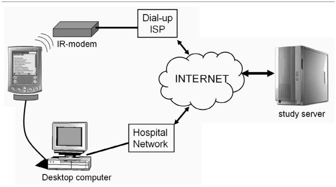
The internet-based data transfer system. Updated information is downloaded to the handheld device from a study server. Connection to the internet can take place via hardwire synchronization with a desktop computer or using infrared (IR) data transmission to a dial-up modem. ISP, internet service provider.
