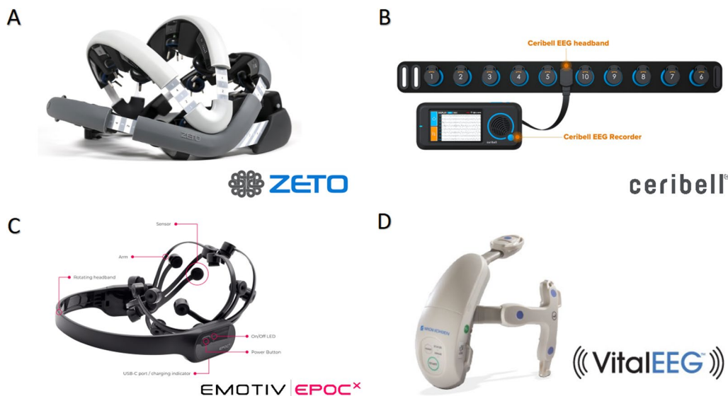
Fig. 4 Rapid Response mobile EEGs— A: Zeto EEG monitoring device that can be worn like a bike helmet and adjusted according to head size. It has 19 electrodes with A1/A2 reference electrodes and 10–20 system complaints. B: Ceribell EEG headband that any healthcare provider can set up rapidly with the pocket-sized Ceribell EEG recorder that provides clinical quality EEG of 10 channel electrodes and on-device EEG. C: EMOTIV EPOC x EEG headset is a 14-channel EEG with a 9-axis motion sensor that can detect head movements. It uses Bluetooth technology to wirelessly transmit data to a computer or mobile device to obtain real-time monitoring of brain activity. D: VitalEEG™ Wireless EEG Headset is a low channel count that can be rapidly deployed by any ER or ICU nurse and remotely monitored by an EEG technologist or physician. Adapted from: https://zeto-inc.com/device/ , https://ceribell.com/ , https://www.emotiv.com/epoc-x/ , https://us.nihonkohden.com/products/vitaleeg-wireless-eeg-headset/
