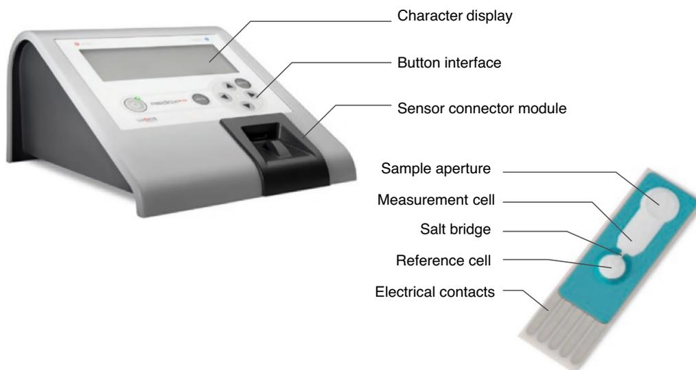
**Fig. 2** Image of the portable RedoxSYS analyzer and disposable strip. From [36] with permission
