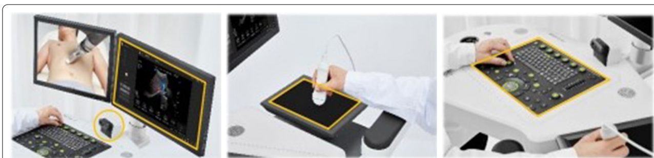
Fig. 2 The figure shows the high-definition audio and video systems equipped on the doctor's side (from left to right), which are used to transmit the doctor's voice and video; the simulated operator system is used to control the robotic arm; the teleultrasound control panel is used to adjust the parameters of the ultrasound machine
