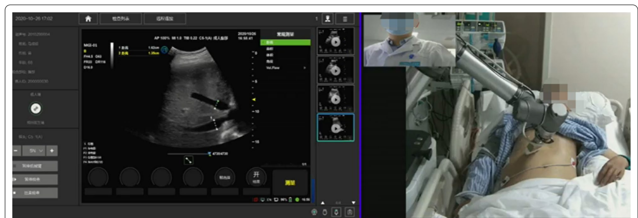
Fig. 5 This is a real-time picture of robot-assisted teleultrasound diagnosis, which displays clearly the real-time transmitted ultrasonic images, the position of the probe on the patient and the patient's status
