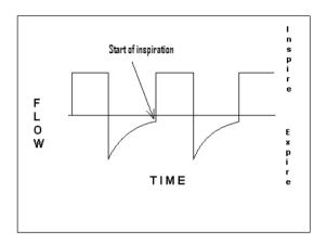
Ventilator tracing with a square wave, or constant flow, pattern. Note that the machine is triggered to initiate a breath before flow returns to zero (the horizontal axis). This indicates that auto-PEEP (positive end-expiratory pressure) is present and directs the clinician to investigate further.
