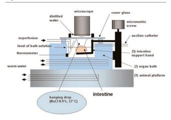
Schematic representation of the cross-section of the tissue platform disclosing the optical way.
