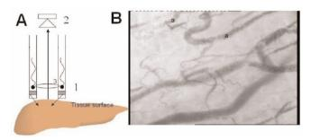
(A) 1, green light-emitting diodes; 2, ccd camera; 3, magnifying lens.(B) Sublingual sidestream dark field image showing arterioles (a) in the microcirculation.
